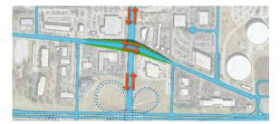
A grade separation between the two roads by depressing Lindbergh and bridging Old Olive overhead.
